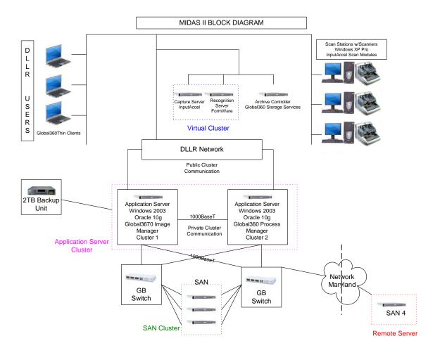
Two identical windows 2003 servers are resident on HP hardware for redundancy. Each server cluster is connected to three LeftHand Network SAN storage devices for data redundancy. The storage devices contain multiple hard disks. Dual iSCSI interface to storage devices on 1000BaseT Channel interface will be used. For interface redundancy dual 1000BaseT interface cards are used.
