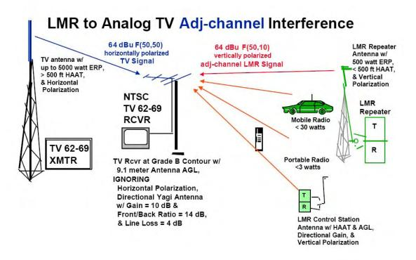
The equivalent ratios for a DTV station's 41 dB F(50,90) desired field strength contour are land mobile 17 dB F(50,10) contour for co-channel and land mobile - 23 dB F(50,10) contour for adjacent channel.
