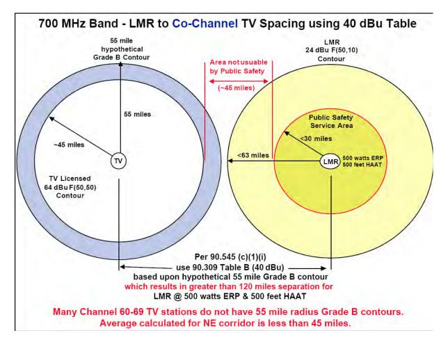
This would permit public safety applicants to take into account intervening terrain and engineering techniques such as directional and down-tilt antennas in determining the necessary separation to provide the required protection. Public safety applicants who use the engineering techniques must consider the actual TV/DTV parameters and not base their study on the 88.5 km hypothetical or equivalent Grade B contour. If land mobile interference contour does not overlap
