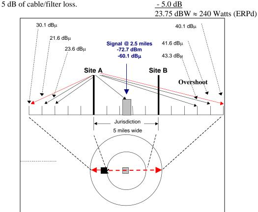
Figure 2 - Field Strength From Left Most Site.
