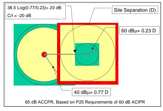
Figure 7 - Example Of Adjacent/Alternate Overlap Criterion
