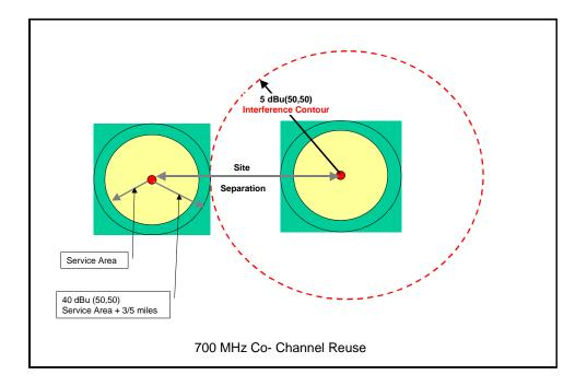
Figure 4 - Co-Channel Reuse Criterion
