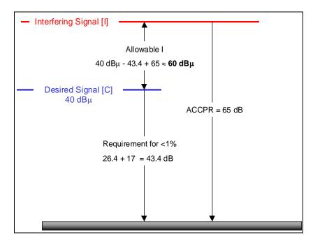
Figure 6 - Adjusted Adjacent 25 kHz Channel Interfering Contour Value
